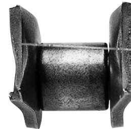
(3) Offset link plate fatigue. Offset link plates are bent at the center, and the resulting concentration of stress at the bend can cause a fatigue break. Avoid using offset links in high-stress applications.
