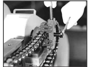
Fig. 5 Cutting chain using a chain breaker
