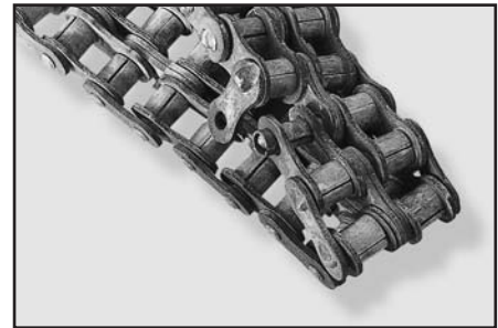
Fig. 31 Corrosion of stainless steel roller chain
