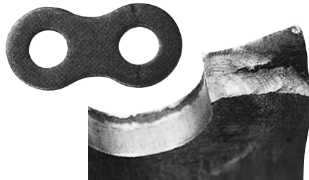
(2) Fatigue fracture. By repeatedly applying a load past its fatigue limit (fatigue strength), the fatigue will start at holes and then suddenly break.
