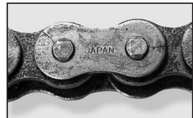
Fig. 32 Hydrogen embrittlement cracking
