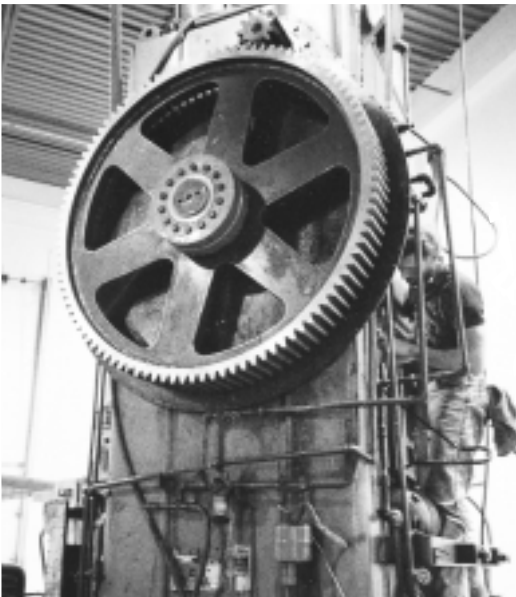
Fig. 41: Shrink Disc® on bull gear of punch press.
