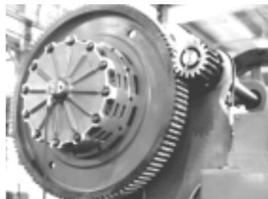
Fig. 6: Pinion Gear Pinion gear and flywheel both mounted with RfN 7012 Locking Assemblies™.
