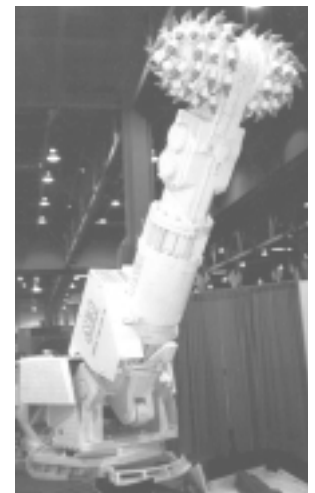
Fig. 7: Cutter Heads Cutter heads fastened with Locking Assemblies™.
