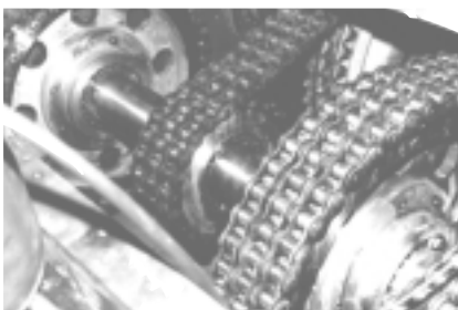
Fig. 4: Sprockets Input shaft for 750 HP draw works showing applications of Locking Assemblies™ and adaptor flanges.
