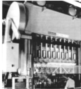
Fig. 33: Gear Gear mounted with a Shrink Disc® on a straight side press.
