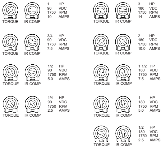
Figure 20. Recommended TORQUE and IR COMP Settings for 174109 Series Controls
