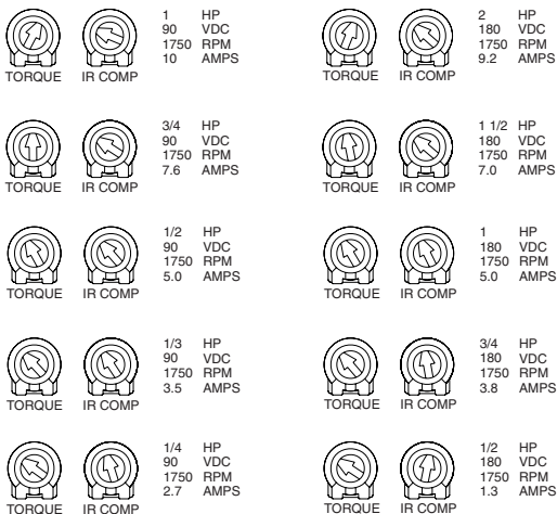
Figure 19. Recommended TORQUE and IR COMP Settings
